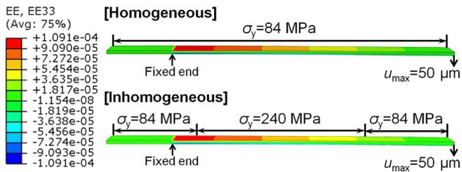
Fig. 4. FEA simulations showing strain variations in homogeneous and inhomogeneous cantilevers at a given displacement  $u_{\max}$ .
