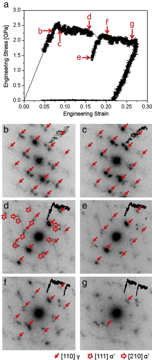
Fig. 3. Results from *in situ* TEM compression test under diffraction mode. (a) Engineering stress–strain curve; (b)–(g) the captured video frames exhibiting diffraction patterns for the points marked on the curve. Note that the martensite spots in (d) are also seen in (e)–(g), but not arrow-marked to avoid complexity.
