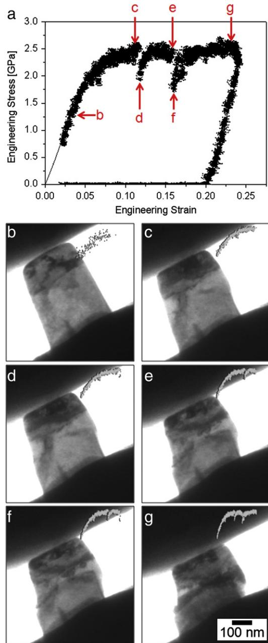
Fig. 4. Results from *in situ* TEM test under bright-field mode. (a) Engineering stress–strain curve; (b)–(g) the captured video frames showing bright-field images for the points marked on the curve.
