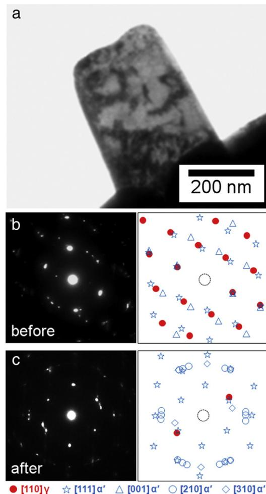
Fig. 2. Representative *ex situ* TEM images. (a) Bright-field image of the nanoplate before compression; (b)–(c) the diffraction patterns taken (b) before and (c) after compression with corresponding schematics.
