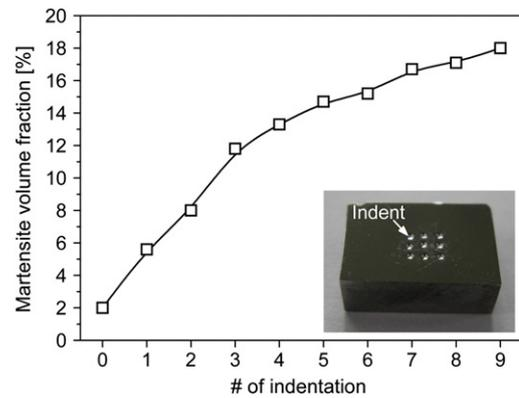
Fig. 1. Change in the estimated martensite volume fraction with increasing number of high-load indentation.
