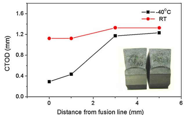
Fig. 2. CTOD change with the precrack location. Inset image shows an example of the regular-shaped precrack of the CTOD specimen.
