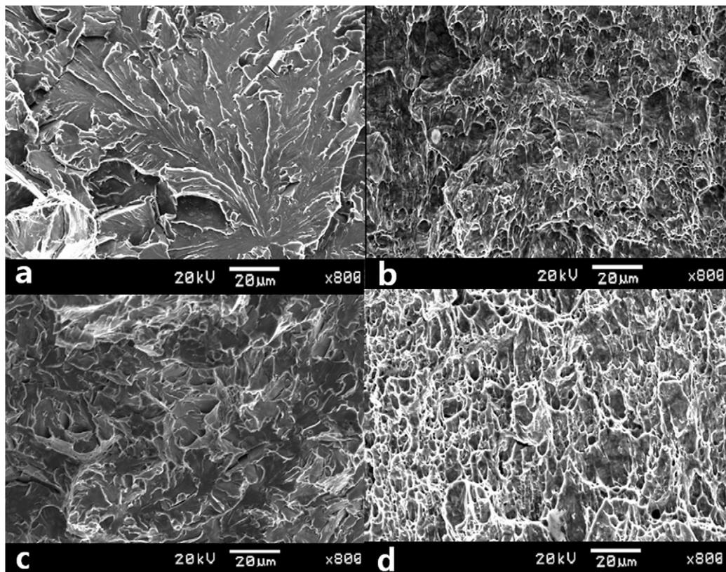
Fig. 6. SEM fractographs of simulated HAZ specimens: (a) IC CGHAZ at  $-40^{\circ}\text{C}$  and (b) RT, (c) FGHAZ at  $-40^{\circ}\text{C}$  and (d) RT.
