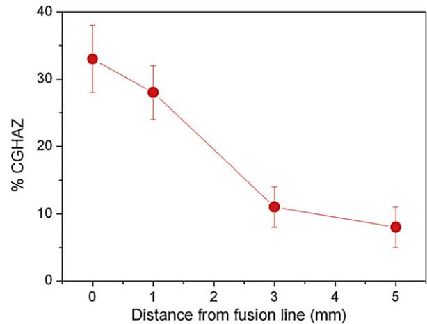
Fig. 4. Fraction of CGHAZ in the precrack tip.
