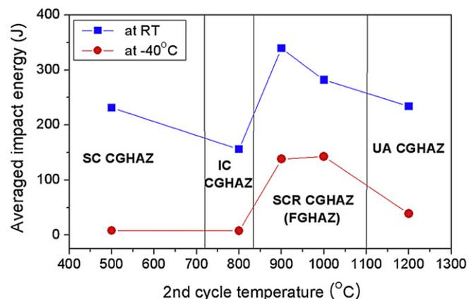
Fig. 5. Change in impact energy of simulated HAZ specimens as a function of the second peak temperature.
