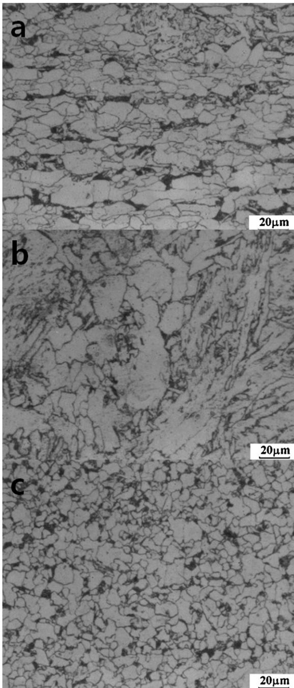
Fig. 3. Microstructural change within HAZ: (a) base metal, (b) CGHAZ region, and (c) FGHAZ region.
