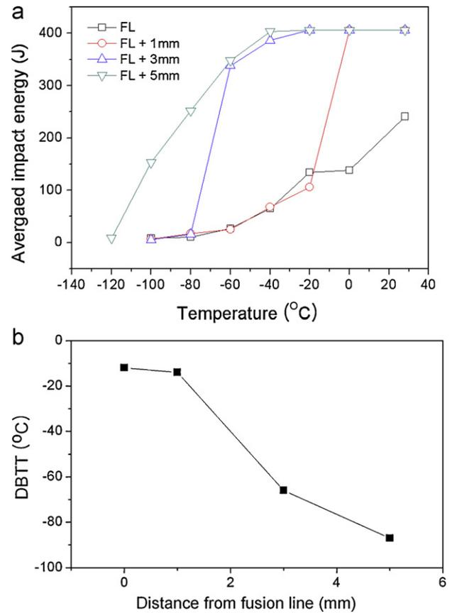
Fig. 1. Results of Charpy impact tests: (a) variation in averaged impact energy as a function of testing temperature; (b) DBTT change with the notch location.
