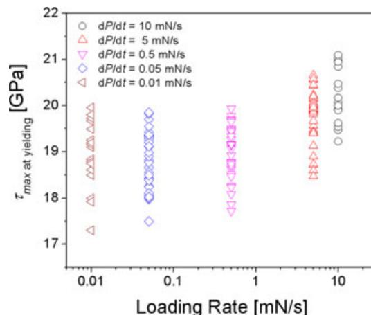
Fig. 3. Variation in the maximum shear stress for the elastic-plastic transition as a function of loading rates.
