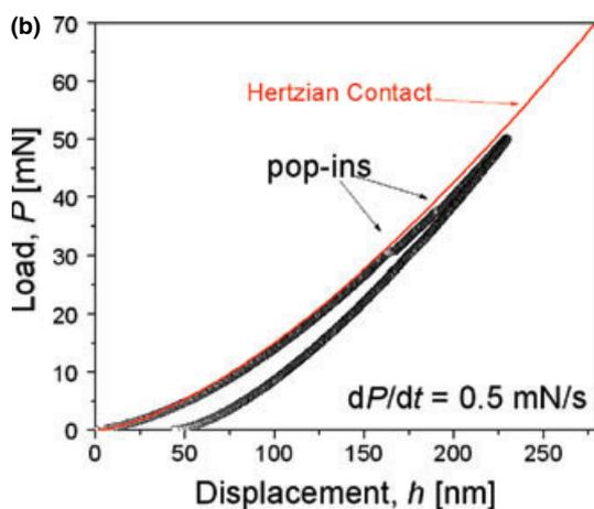
Fig. 1. Nanoindentation load-displacement curves showing (a) perfectly elastic behaviors below the first pop-in load; and (b) pop-in during loading and permanent deformation after unloading.
