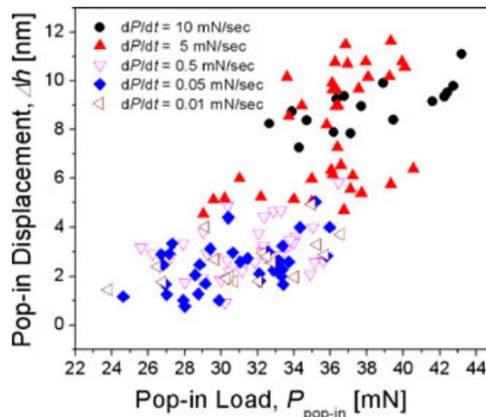
Fig. 2. The relationship between the load at the first pop-in and the resulting displacement excursion during the pop-in.
