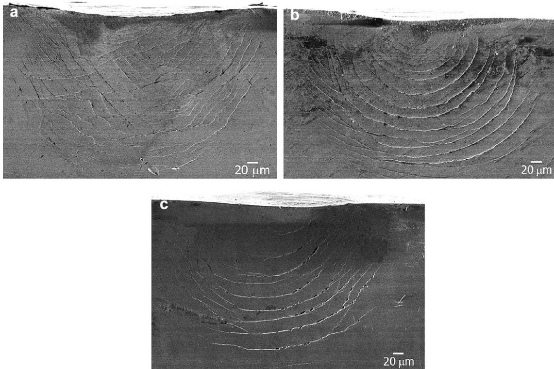
Fig. 2. Optical micrographs showing the development of subsurface deformation underneath the macroscopic spherical indentation made at  $P_{\max} = 196$  N; (a) as-cast, (b) 50 h-charged, and (c) 100 h-charged sample.
