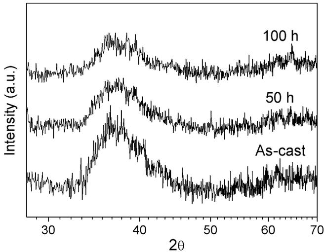
Fig. 1. XRD patterns of as-cast and hydrogen-charged specimens.
