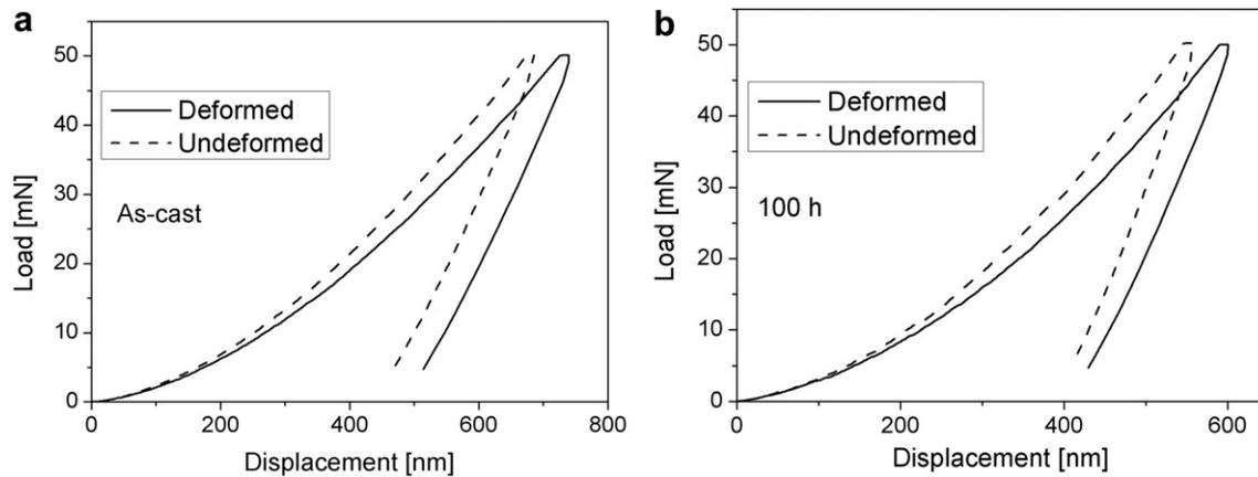
Fig. 3. Representative  $P$ - $h$  curves obtained at the peak-load of 50 mN and constant strain rate of 0.1/s; (a) as-cast and (b) 100 h-charged sample.
