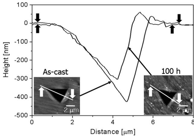
**Fig. 6.** Typical example of AFM analysis of the nanoindentation impression made in the undeformed region.
