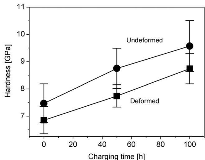
Fig. 5. Summary of the change in nanohardness as a function of hydrogen charging time.
