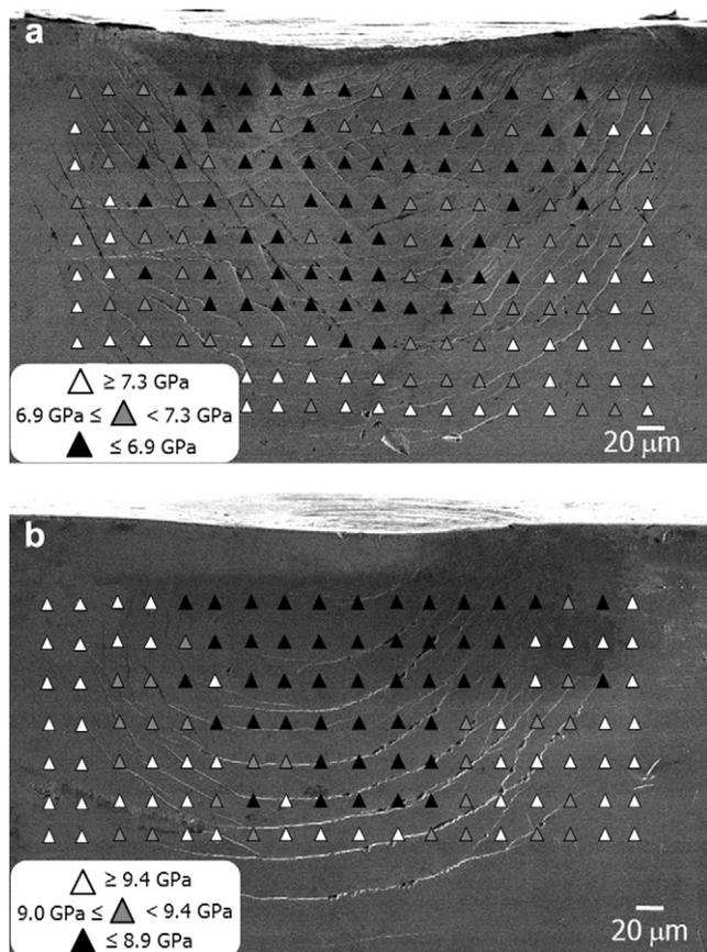
Fig. 4. Nanohardness distribution map in the subsurface deformation region; (a) as-cast and (b) 100 h-charged sample.
