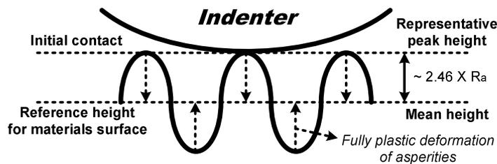
Fig. 1. Schematic of rough-surface model.
