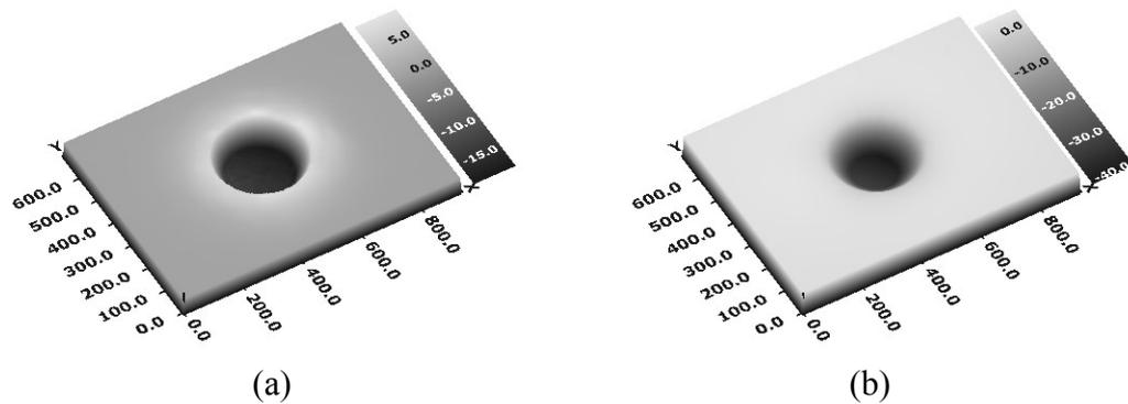
Fig. 2. Residual indents measured by optical profiler for (a) W (pile-up) and (b) Ni (sink-in).
